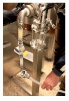
Quick disconnects from CPC are used to connect fluid and air lines in the brewing process at Urban Growler Brewing Co.
