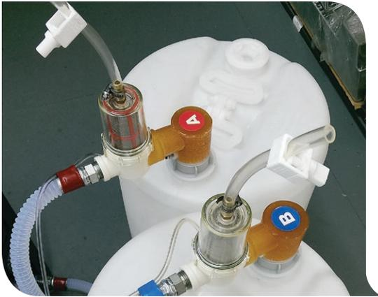
A-type and B-type chemicals are supplied in bulk containers with pre-installed single-use dip-tube assemblies.
