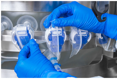
Step 1 - Connect the Aseptic Connector to the matching Aseptic Connector on the SUT
