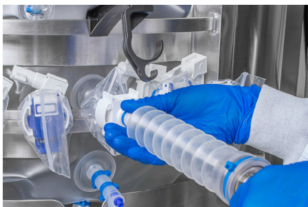
Step 3 - Pull tabs and line up probe for insertion
