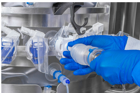
Step 4 - Compress the bellows and probe to complete aseptic insertion
