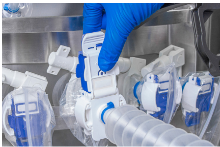
Step 2 - Connection of the probe to the SUT
