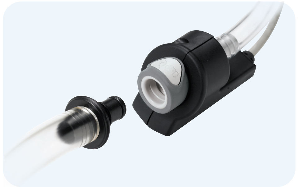
Data-transmitting fluid connectors include two parts: the coupling body (right), which houses an RFID reader, and the coupling insert (left), which houses an RFID tag. The reader can read and write information on the tag. Illustration depicts an IdentiQuik® non-spill coupling from CPC.
